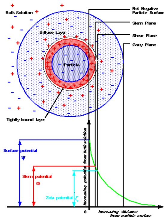
**Figure 1.** Schematic illustration of electrical double layer (EDL).
